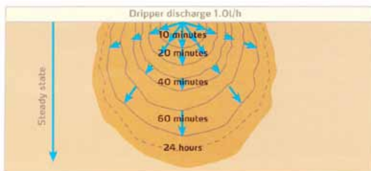
Typical wetted soil volume following a one-hour irrigation
